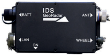
Radar Control Unit
